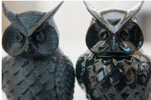
Rysunek 10 – A 3D printed object, before and after vapour smoothing. Source: www.geeetech.com
